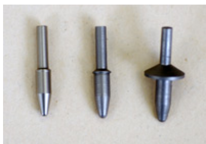
10-Meter air rifle and pistol scoring gauges, l. to r., Air Rifle/Pistol Inward, Air Rifle Outward and Air Pistol Outward. Note the small flange on the inward gauge and the larger flanges on the outward gauges. The gauges shown here are all Gunsmithing, Inc. gauges.
